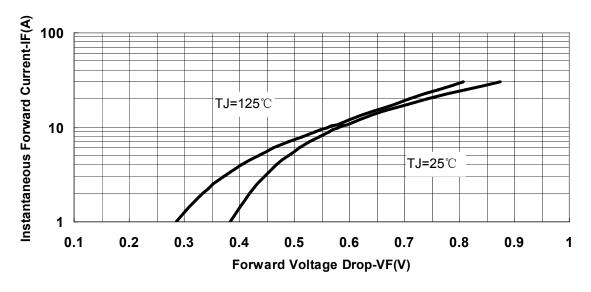
Fig.3-Typical Instantaneous Forward Voltage Characteristics
