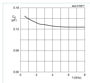
Fig. 5. Diode capacitance as a function of frequency; typical values
