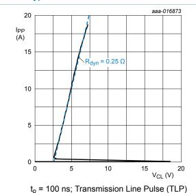
Fig. 7. Dynamic resistance with positive clamping voltage
