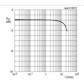
Fig. 6. Insertion loss; typical values
