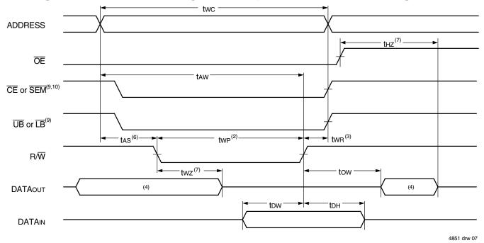
Timing Waveform of Write Cycle No. 2, CE Controlled Timing<sup>(1,5)</sup>
