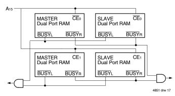
Figure 3. Busy and chip enable routing for both width and depth expansion with IDT70V37 RAMs.
