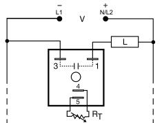
Load may be connected to terminal 3 or 1.
