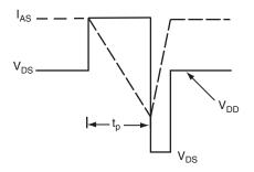
Fig. 12b - Unclamped Inductive Waveforms
