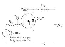
Fig. 10a - Switching Time Test Circuit
