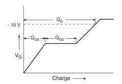
Fig. 13a - Basic Gate Charge Waveform
