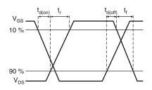
Fig. 10b - Switching Time Waveforms
