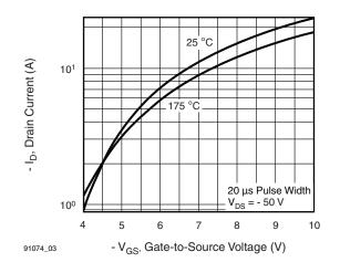
Fig. 3 - Typical Transfer Characteristics
