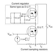
Fig. 13b - Gate Charge Test Circuit
