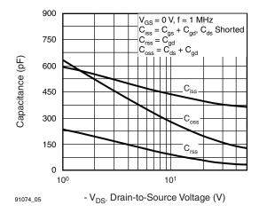
Fig. 5 - Typical Capacitance vs. Drain-to-Source Voltage
