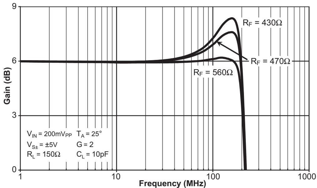
Figure 3 Gain of 2 small signal bandwidth
