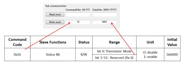
Press [Write Word] to enable Thermistor
